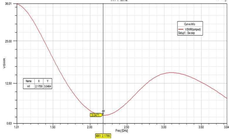
Fig 12: Return loss of the antenna using micro strip line feed method is -5.9443dB at 2.17GHz which is not very optimal.
