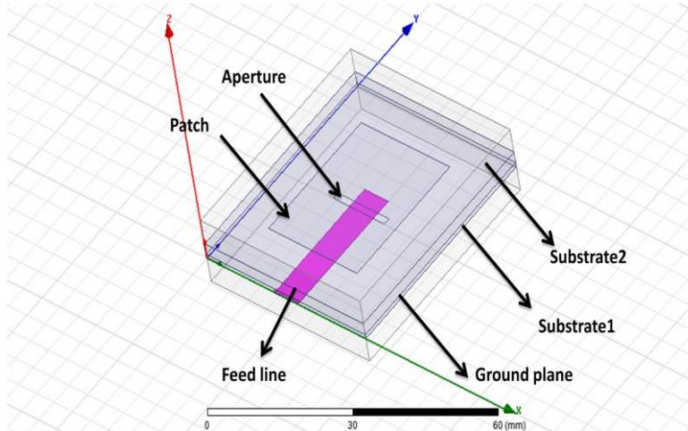
Fig 11: Designed model of Aperture coupled feed method in HFSS software
