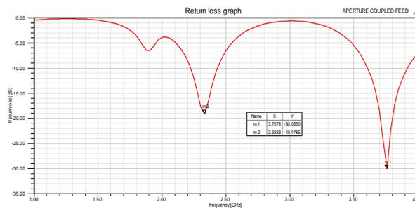
Figure 7.13: Return loss of the antenna using aperture coupled feed method is -30dB at 3.75GHz which is very much better value.
