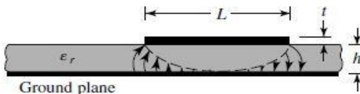
Fig 2: Side view of Microstrip patch antenna
