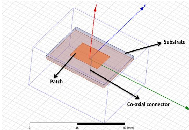
Fig 9: Designed model of Coaxial feed method in HFSS software
