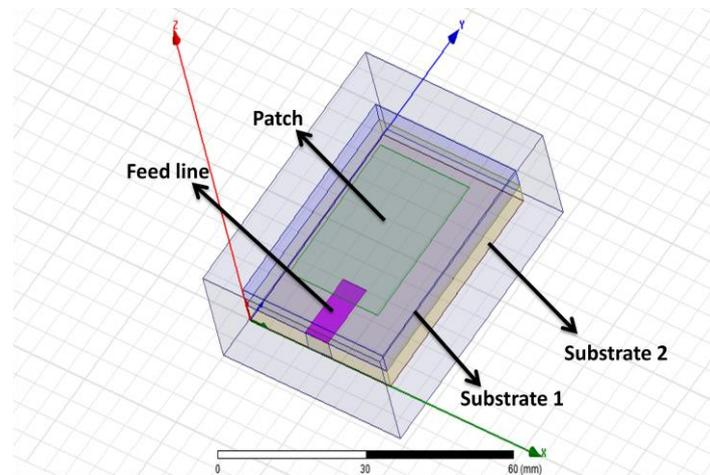
Fig 10: Designed model of Proximity coupled feed method in HFSS software
