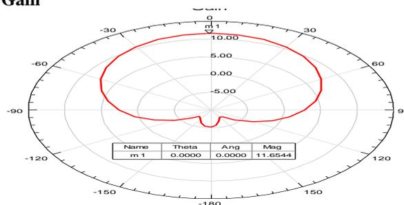
Figure 7.15: Radiation pattern of aperture coupled feed technique.
