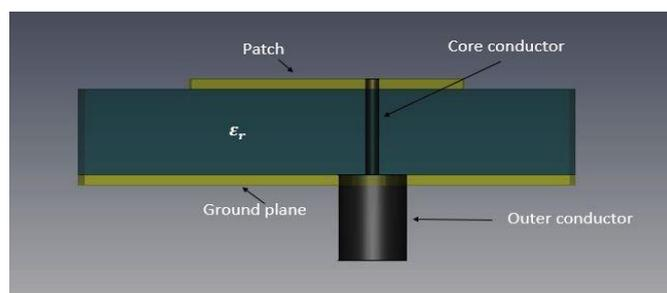
Fig 5: Coaxial probe feed
