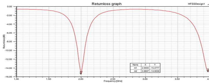
Fig 20: Return loss of the antenna using Proximity coupled feed method is -15.477dB at 2GHz which is very much better value.
