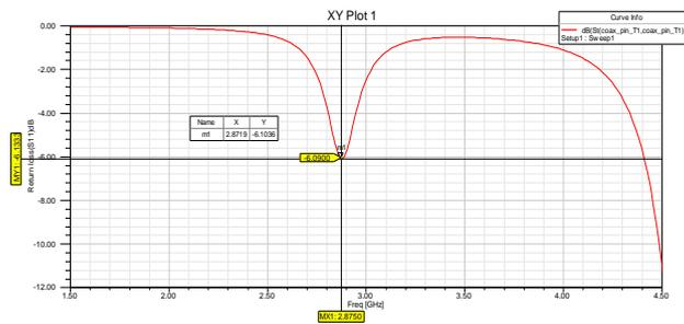
Fig 16: Return loss of the antenna using coaxial feed technique is -6.103dB at 2.87GHz which is not very optimal.
