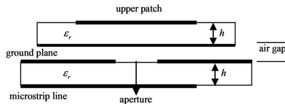
Fig 7: Aperture coupled feed
