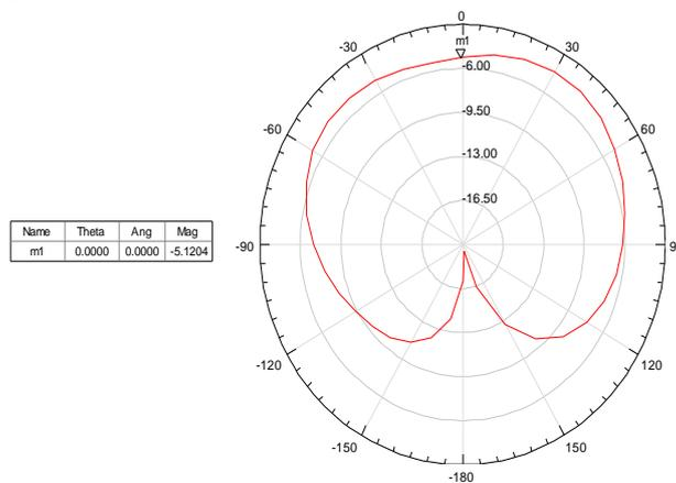
Fig 14: Radiation Pattern Of Microstrip Line Feed Method
