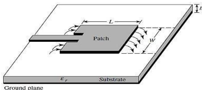
Fig 1: Top view of Microstrip patch antenna
