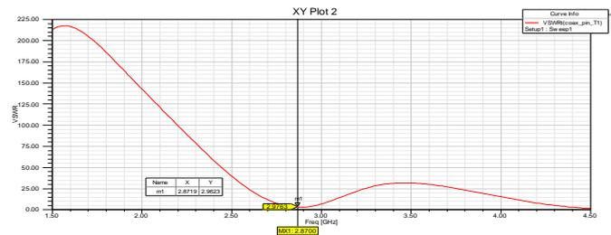
Fig 17: VSWR of Coaxial feed technique is 2.9623 at 2.87GHz.
