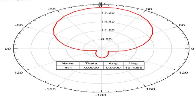
Fig 22: Radiation pattern of proximity coupled feed technique.
