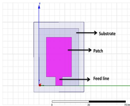
Fig 8: Designed model of Microstrip line feed method in HFSS software
