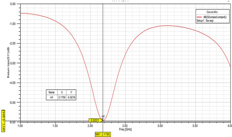
Fig 13: VSWR of Micro strip line feed technique is 3.0471 at 2.17GHz.
