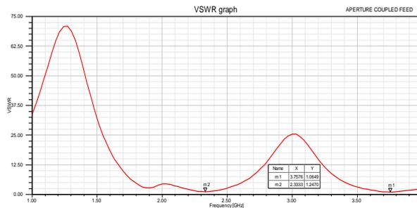
Figure 7.14: VSWR of Aperture Coupled feed technique is 1.06 at 3.75GHz.
