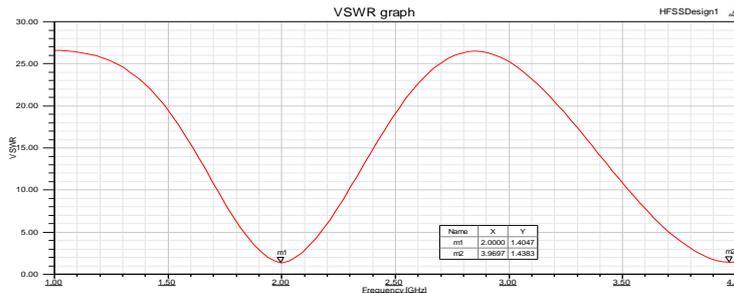
Fig 21: VSWR of Proximity Coupled feed technique is 1.4 at 2GHz
